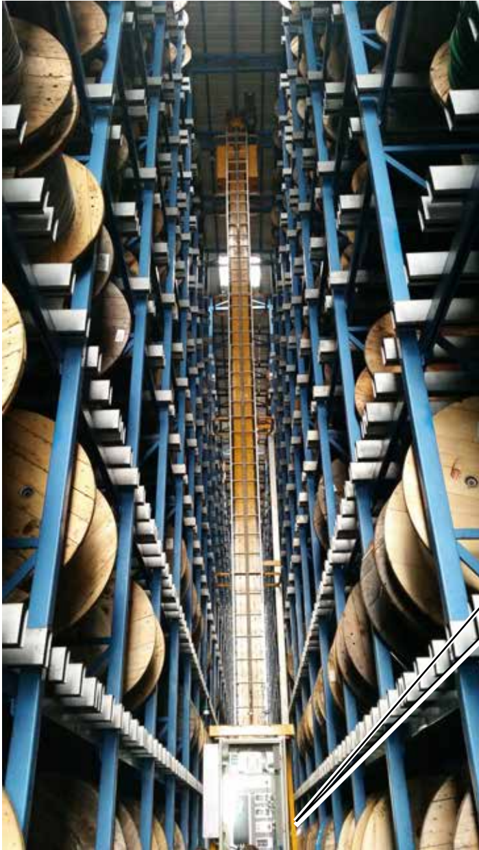
Fig. 6 - SADA cable warehouse in Fiorano (made by System Logistics. - 1000 place max 2500 kg.
