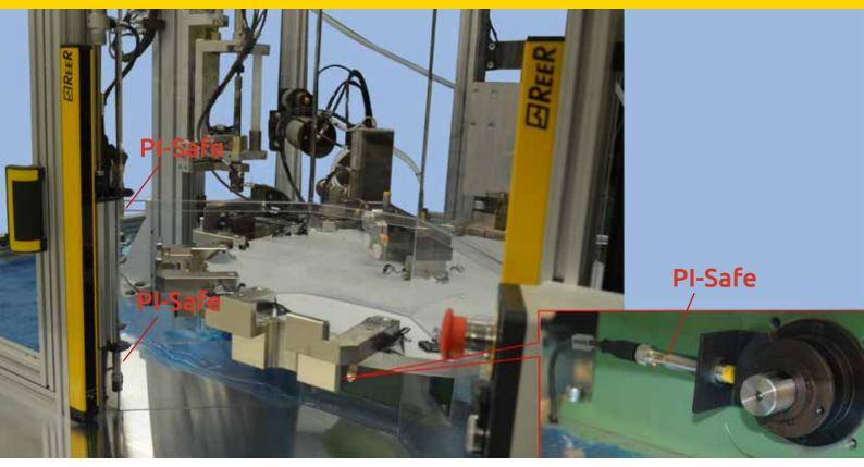
The position monitoring of the protection screen and rotary table are carried out by means of inductive safety sensors PI-Safe M12.
