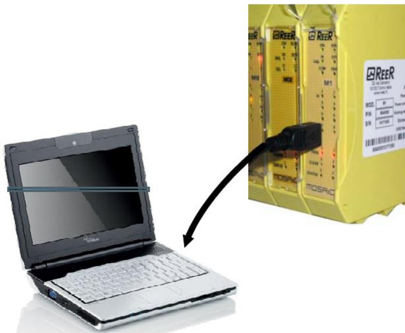
Figure 2: Programming tool connection via USB2.0 to MOSAIC-Series
