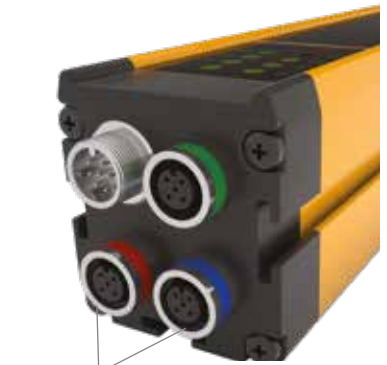
Muting sensor connectors (M12 5-pole)
